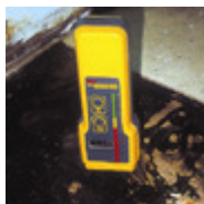
Measuring moisture levels of a subfloor. (photo, Terry Brennan)
