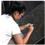
Clear plastic tape is used to collect a sample. The sample is analyzed with a microscope to determine whether the substance is mold or soot. (photo, Terry Brennan)
