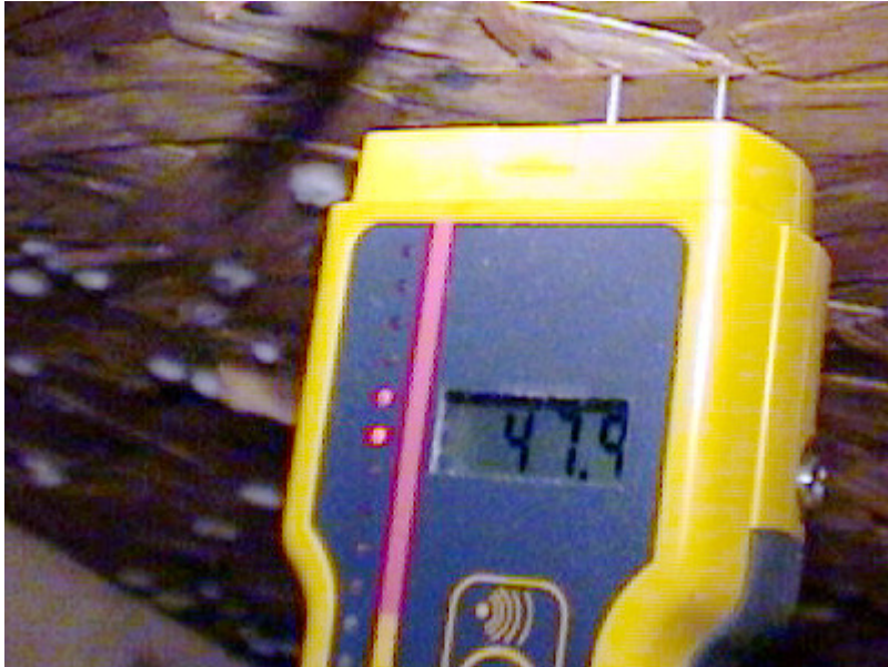
Measuring moisture levels of a subfloor. (photo, Terry Brennan)
